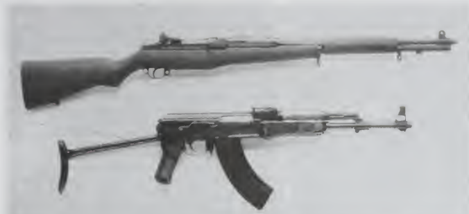
Figure 12: Two autoloading infantry rifles of the 20th century. (Top) The U.S. M1, a gas-operated semiautomatic. (Bottom) The Soviet AK-47, a gas-operated assault rifle.
